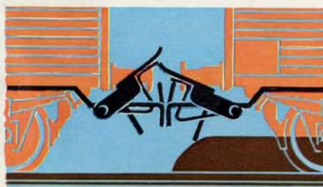
Raising the ramps releases the coupling.
