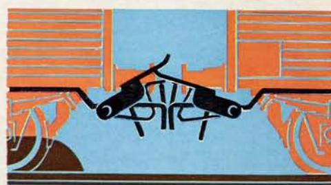
This design of coupling allows a train to be shunted further after the uncoupler has operated, without the couplings re-engaging.
