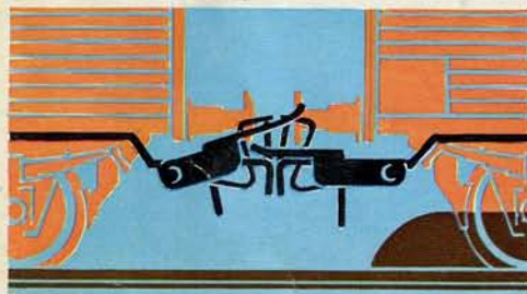
Raising the ramps releases the coupling.
